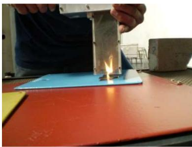
Figure 5-7. Laser Stripping Blue Coated Panel
