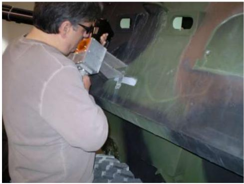
Figure 4-4. LAV Surface after Stripping
