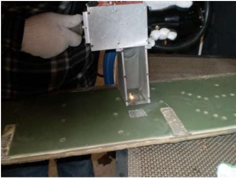
Figure 4-7. Stripping Humvee Front Plate
