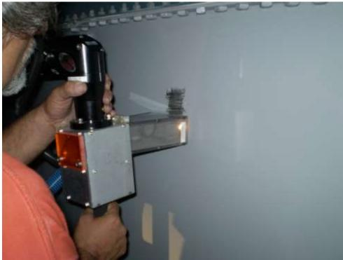
Figure 3-7. Laser Stripping Coating
