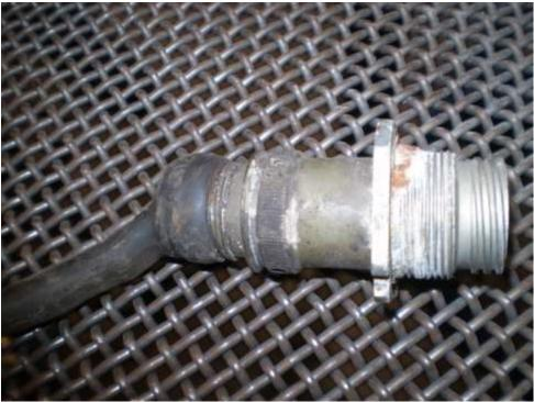
Figure 4-14. Electrical Plug after Stripping
