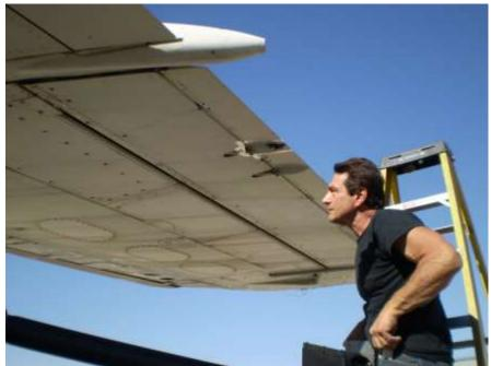
Figure 2-11. Aileron after Stripping
