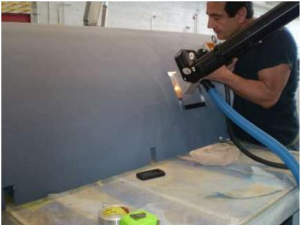
Figure 2-5. Cowling Being Stripped
