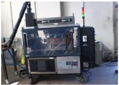
Figure 5-1. Laser Stripping Device at Navy Maintenance Center
