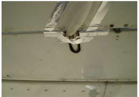
Figure 2-10. Aileron Taped Off
