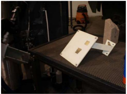
Figure 4-15. Anodized Aluminum Part after Stripping
