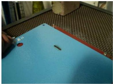
Figure 5-8. Blue Coated Panel after Stripping
