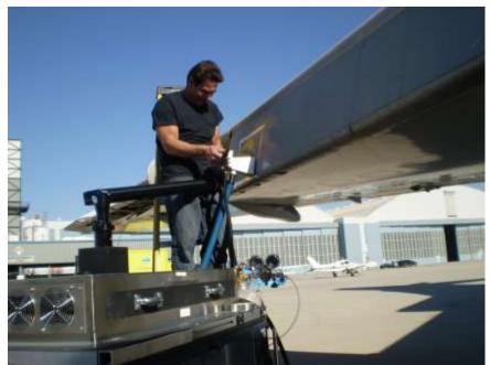
Figure 2-8. Krueger Flap Being Stripped
