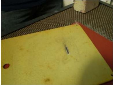
Figure 5-9. Yellow Coated Panel after Stripping
