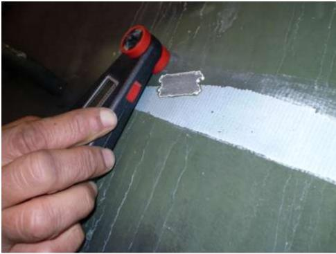
Figure 4-5. LAV Close-up after Stripping CARC and Tape.
